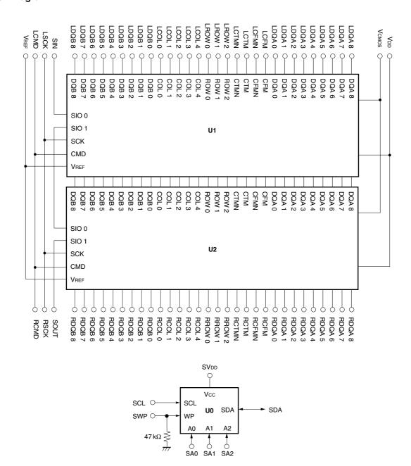
**Remarks 1.** Rambus Channel signals form a loop through the RIMM module, with the exception of the SIO chain.
