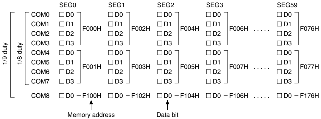
Fig. 4.7.4.1 Correspondence between display memory and LCD dot matrix
