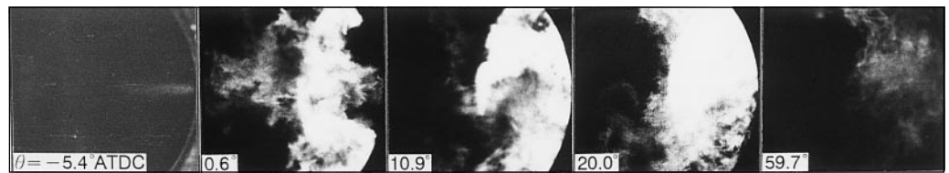
Direct flame image (photographed with high-speed camera)
