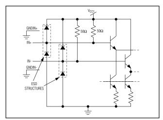
Figure 2. CML Input Equivalent Circuit
