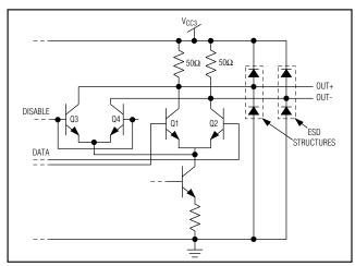
Figure 3. CML Output Equivalent Circuit
