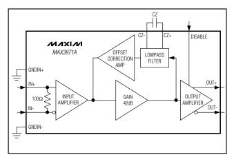
Figure 1. Functional Diagram
