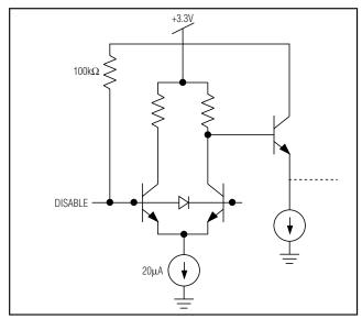
Figure 4. TTL Input Stage
