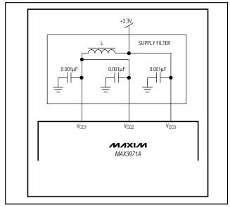
Figure 5. Power-Supply Filter
