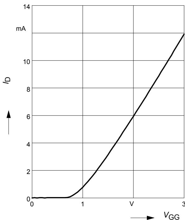
**Drain current  $I_D = f(V_{GG})$**
