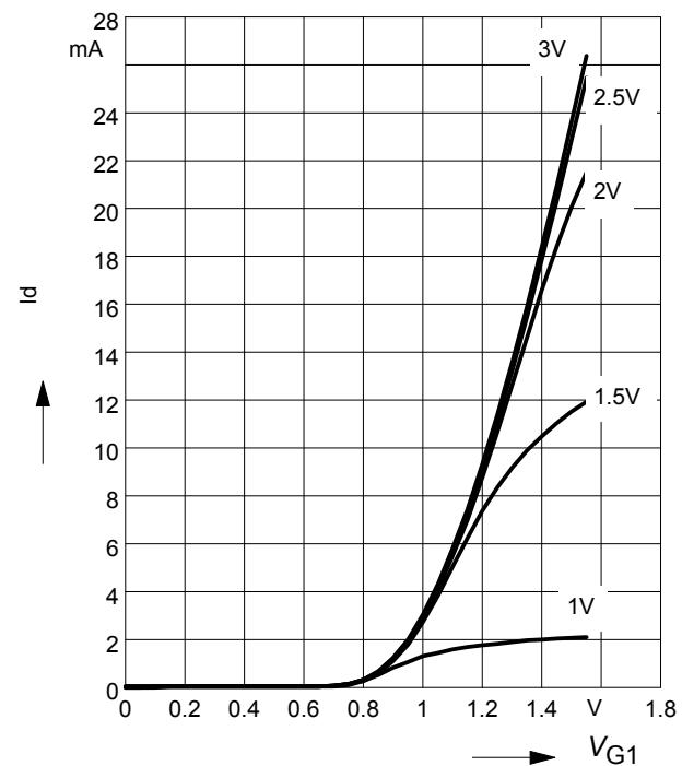
**Drain current  $I_D = f(V_{GG})$**
