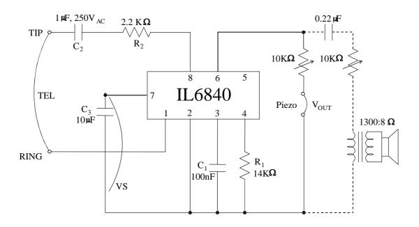
$$f_1 = 3.22 \, \bullet 10^4 \, / \, R_1 \, (K\Omega); \quad f_2 = 5/7 \, \, f_1; \ \, f_{sweep} = 1000 \, / \, C_1(nF)$$
