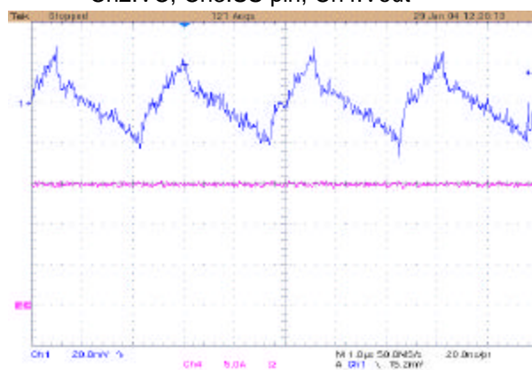
Figure 17 - Output Voltage Ripple @ 15A Ch1:Output, Ch4:lout (5A/Div)
