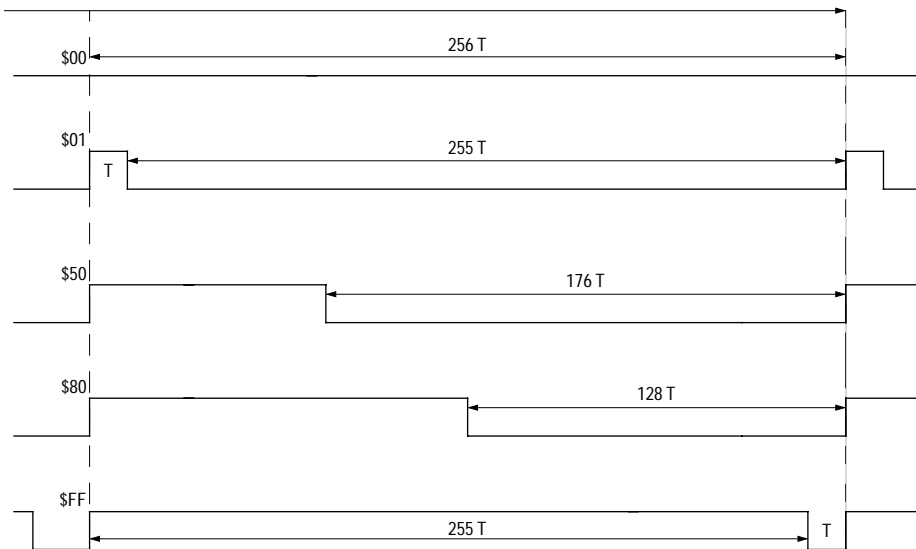
Figure 12-2 PWM output waveforms (POL = 1, active high)
