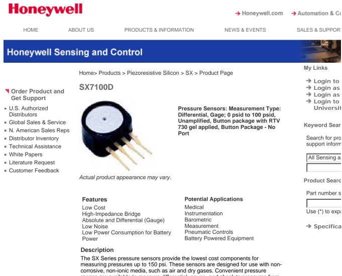
ranges are available to measure differential, gauge, and absolute pressures from 0 psi to 1 psi (SX01) up to 0 psi to 150 psi (SX150).
