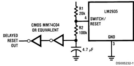
**FIGURE 5. Reset Pulse on Power-Up
