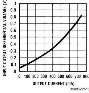
**Dropout Voltage ( $V_{STBY}$ )**
