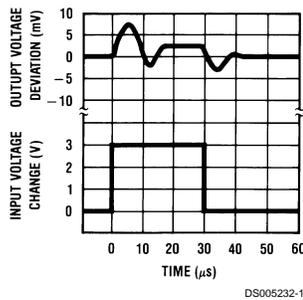
**Load Transient Response ( $V_{OUT}$ )**
