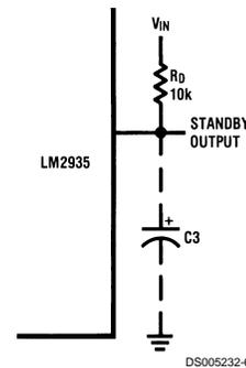
FIGURE 3. Disabling Standby Output to Eliminate C3
