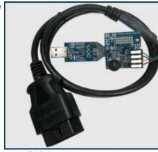
OBD-II standard SAE J1979. These modes allow the OBD Reader to access the current c show freeze frame data, and show the stored diagnostic trouble codes. The purpose of the reference design is to demonstrate an automotive Silicon Labs MCU interfacing to a vehic with a very simple and straightforward design. The MCU communicates with the vehicle u the CAN bus at 500 kbps and does not require an external crystal.
